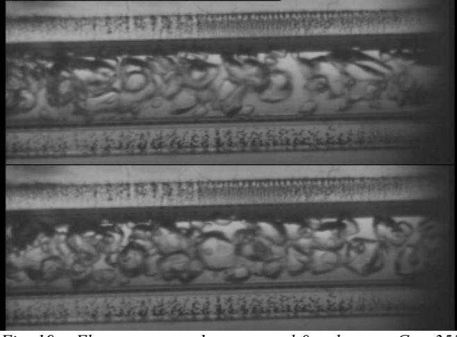
Fig. 19 – Flow pattern at 1-g, top, and 0-g, bottom, G = 355 \text{ kg/m}^2\text{-s} , \Delta T_{sub,in} = -25.3 \text{ K} , and p = 1.8 \text{ bar} , D = 4 \text{ mm} (intermediate heat flux)
