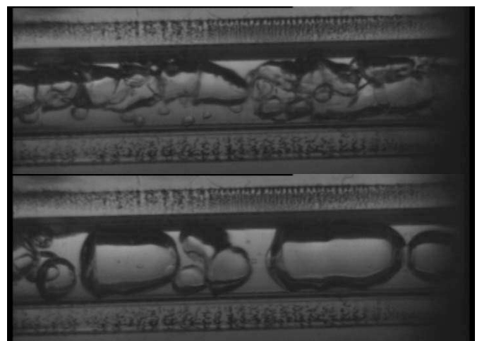
Fig. 18 – Flow pattern at 1-g, top, and 0-g, bottom, q'' = 23800 W/m 2 , x_{out} = 0.066 , D = 4 mm (low mass flux)
