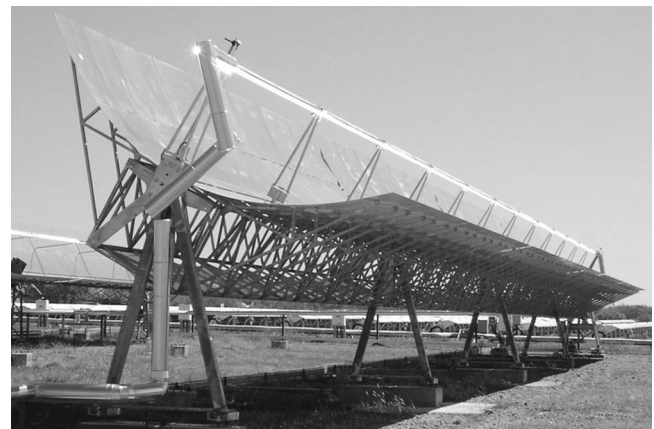
Fig. 5 The EuroTrough collector prototype under test at PSA (Source: PSA)
