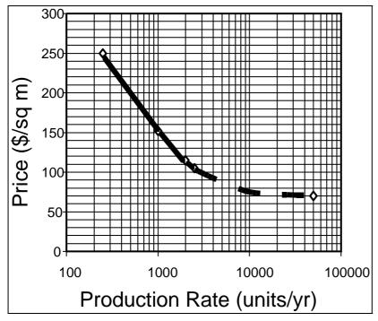
Figure 6.7 Heliostat price as a function of annual production volume. These prices apply to a heliostat with a surface area of 150  $m^2$  and is similar in design to those tested at Sandia National Laboratories. Solid portion of curve is based on estimates by USA manufacturers. Dashed portion is a reasonable extrapolation.
