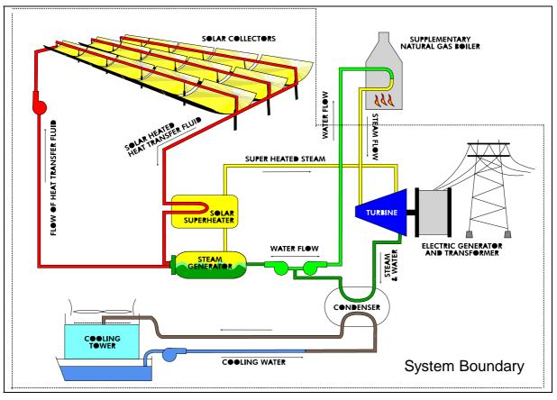
Figure 3.1 Schematic of a SEGS power plant built by LUZ International. Synthetic oil is heated to 390°C within a vacuum-jacketed pipe located at the focal line of a parabolic trough. The hot oil is delivered to a steam generator and returned to the solar field at a temperature of 290°C. The plant can run solar-only, but a fossil boiler is also installed to allow plant operation at night or during poor solar conditions.
