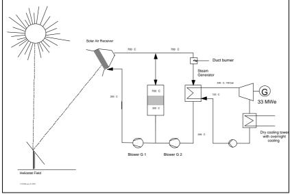
Figure 3.3 PHOEBUS 1B Cycle with Storage
