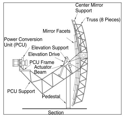
Figure 3.8 The 25 kW dish-Stirling system manufactured by MDA and marketed by Stirling Energy Systems (USA). Dish systems track the sun on two axes and focus direct normal solar insolation on a receiver. The receiver transfers the heat to the engine which converts the thermal power to mechanical power. A generator or alternator converts the mechanical power to electricity. Waste heat is rejected from the engine to the atmosphere.
