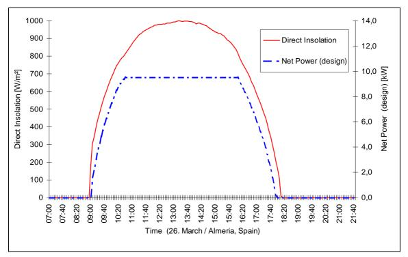
Figure 3.15 Design daily input/output curve for the 10 kWel pre-commercial dish-Stirling unit
