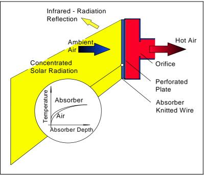
Figure 3.4 Functioning principle of the PHOEBUS Hot Air Receiver
