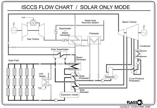
Figure 6.4 Schematic of the Integrated Solar Combined Cycle System (ISCCS) as proposed by Luz International Ltd., Flachglas Solartechnik GmbH, ABB and Tenenge in 1991 to CEMIG for implementation at the Januária site [Courtesy of Pilkington Solar International, Cologne]
