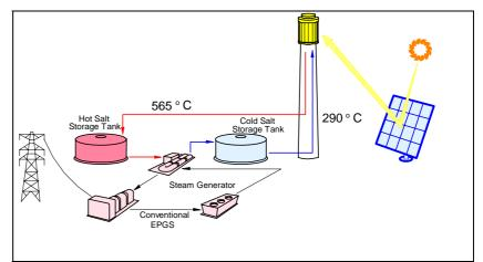
Figure 3.2 Schematic of a molten salt power plant. Molten salt is heated to  $565^{\circ}$ C within a tubular type receiver and pumped to the hot storage tank. When power is needed to meet the load demand on the grid, salt is extracted from the hot tank to a steam generator. The steam drives a conventional electric power generating system (EPGS). After making steam, molten salt at 290°C is returned to the cold tank and pumped back to the receiver.
