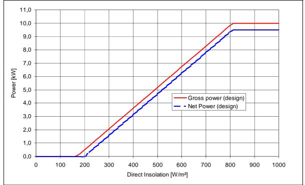
Figure 3.14 Design input/output for the 10 kWel pre-commercial dish-Stirling unit
