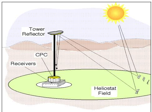
Figure 4.1 Solar 'Tower Reflector' Central Receiver plant concept
