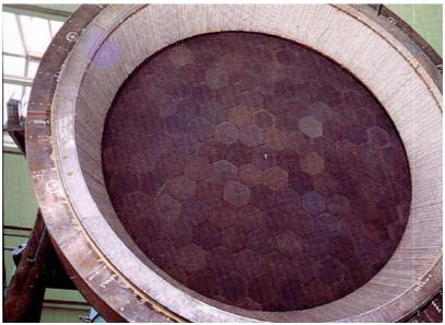
Figure 3.5 View of the 2.5MWt TSA Pilot Receiver during fabrication
