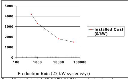
Figure 3.9. Installed cost of a 25 kW MDA dish-Stirling as a function of annual production volume [1].
