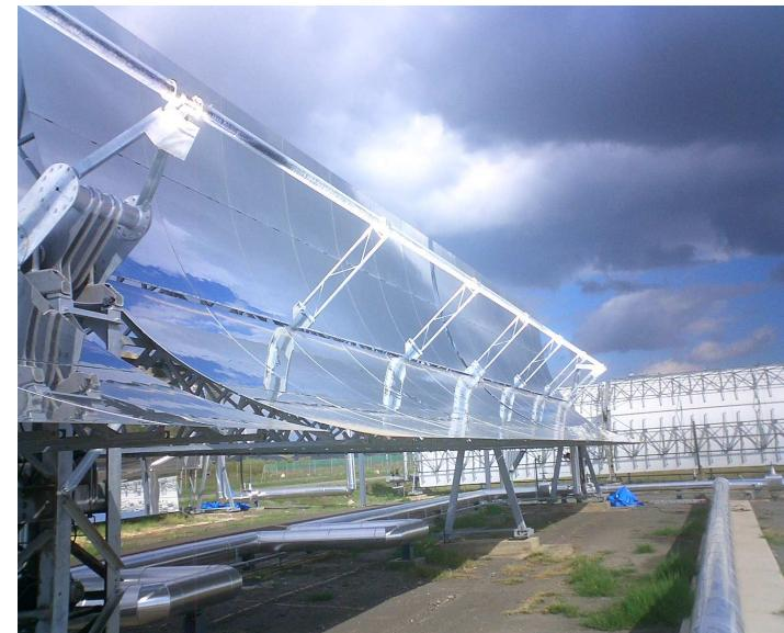
PT with gas test loop in operation
