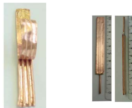
Figure 5- Micro heat pipes manufactured at NCTS.
