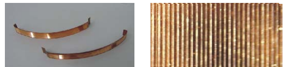
Figure 2- Grooved plates, resulting from the machining process.
