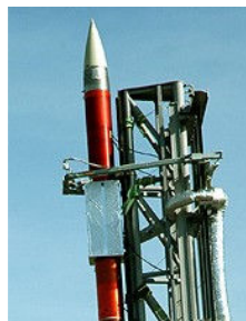
Figure 9: External cooling system.
