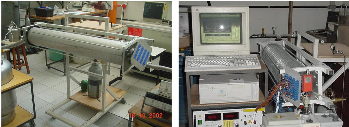
Figure 4.15. Vacuum chamber (left) and experimental setup (right).
