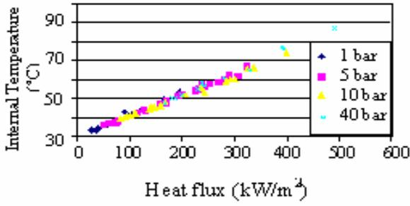
Figure 3: Pressure vessel internal temperature as function of the heat flux
