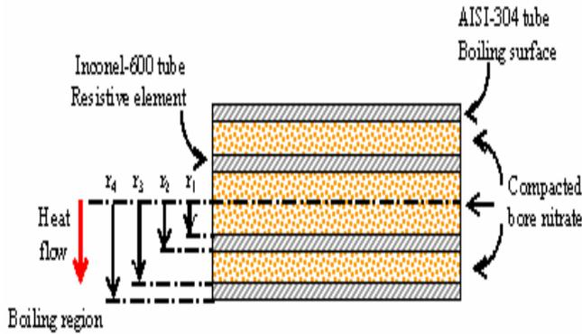
Figure 2: Sketch of the electric simulator.
