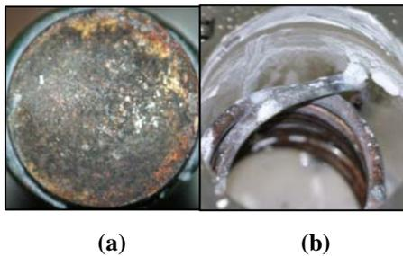
Figure 5 – Images from: a) the heating surface and b) the serpentine condenser, after boiling experiments
