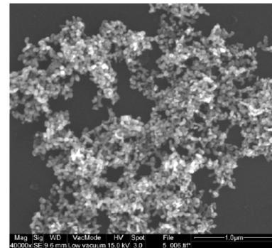
**Figure 3 – Tunnel-Electron-Microscopy of nanoparticles of  $Al_2O_3$**
