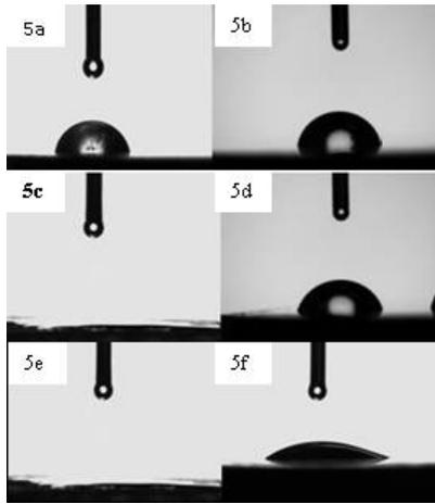
**Figure 8: Contact angles for: a) clean surface, b) rough surface, c-) Alumina deposited surface, d-) Alumina deposited surface after excess removal, e-) Maghemite deposited surface, f-) Maghemite deposited surface after excess removal**
