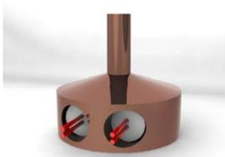
**Figure 2 - Heated part without the teflon cover. The top is discerned to the bottom of the chamber of Fig. 1.**
