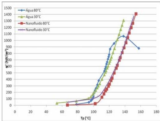
Figure 4 – Partial boiling curves for  $Al_2O_3$ .
