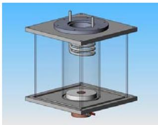
**Figure 1 – Transparent boiling chamber with the heater and the cooling units.**
