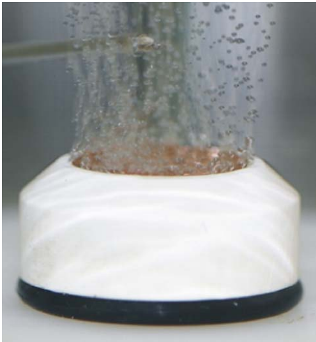
Fig. 3 FC-87 nucleate boiling, q = 30 \text{ kW/m}^2 , T_w = 42.5^\circ\text{C}
