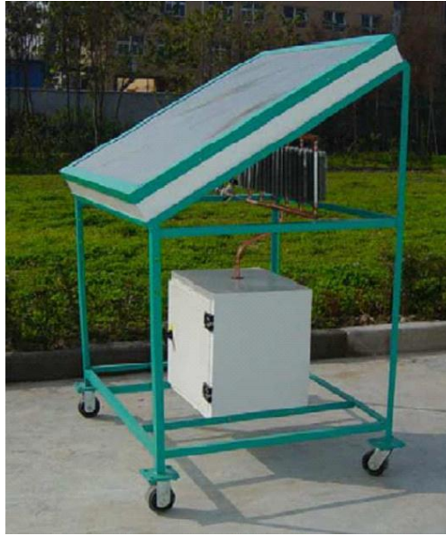
Figure 10. No valve solar ice maker [76].
