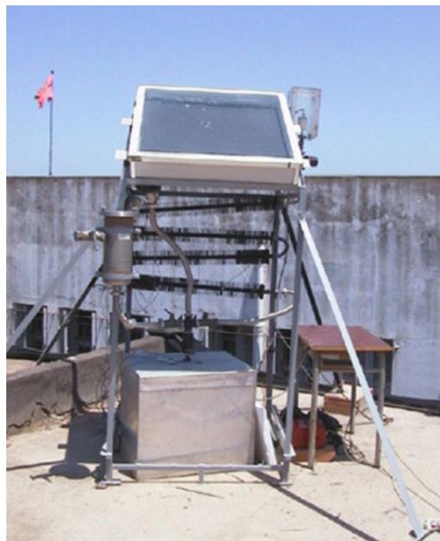
Figure 11. Solar refrigerator tested in Rabat, Morocco [77].
