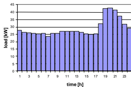
Figure 6: Average daily load curve of the Araras, RO grid (Rüther and Montenegro 2000) during July to September 2002. The average load is 27 kW (equivalent to about 650 kWh/day).
