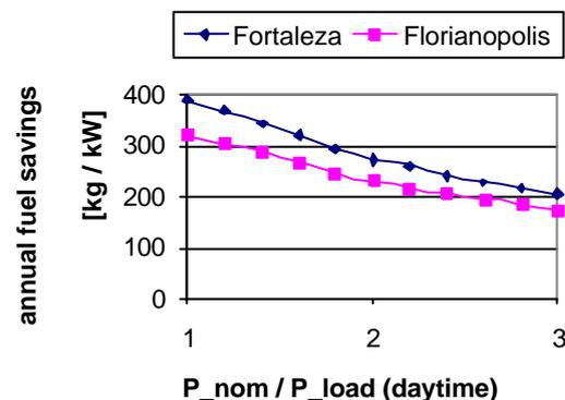
Fig. 4: Same presentation as figure 3a, but for a constant PV-size ( $P_{stc}/P_{load} = 1$ ) and a variation of the nominal capacity of the DGS. Due to the requirement of a minimum load for the DGS (here 0.15  $P_{nom}$ ) the fuel savings are reduced remarkably by the increase of the nominal power.
