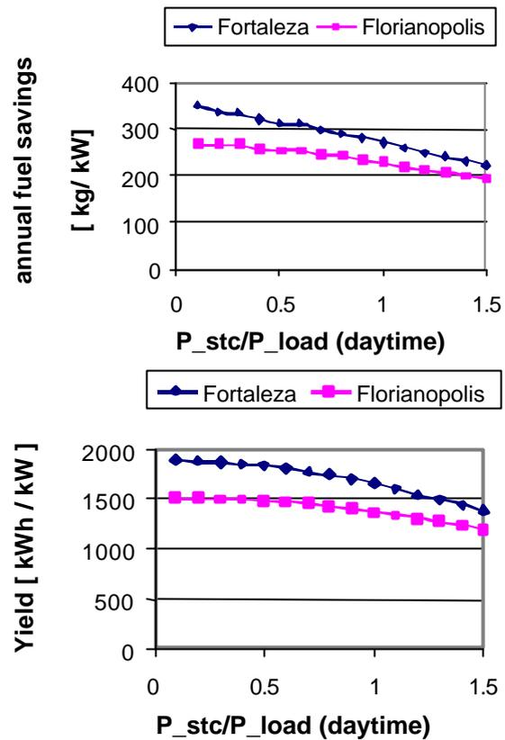
Fig. 3: Results of simulation runs for the specific fuel savings (3a, upper figure) and the yield (3b, lower figure) for PV generators in PV-Diesel Systems without storage as function of the size (STC-power) of the the PV generator, normalized by the average load during daytime. The meteorological conditions of Florianópolis and Fortaleza are used as input. The examples given refer to systems with a DGS with a nominal capacity of twice the average daytime load.
