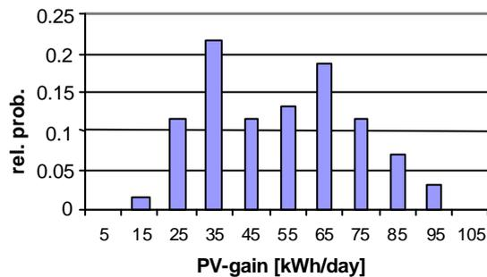
Fig. 8: Distribution of the daily energy gain of the PV-generator at Araras for the period inspected. Taking the effective rating of the PV generator (see text) these gains represent a performance ratio of 0.84.
