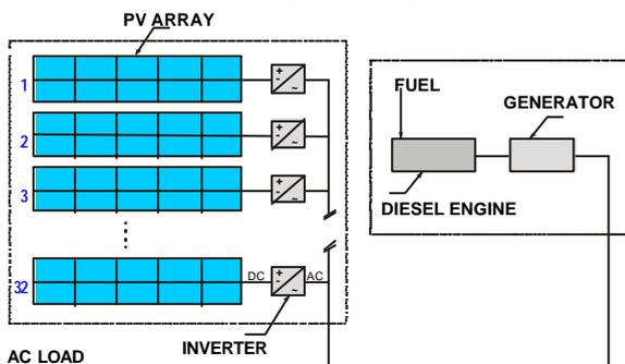
Figure 5 Schematic diagram of the Diesel / PV system without storage currently in operation at Araras, Rondonia (Rüther et al. 2000).
