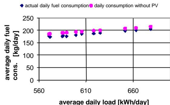
Fig.10: Monthly averages of the daily fuel consumption as given by measured data (diamonds) and estimated values (dots) for a system without PV. The PV gives a 5.5% reduction of the fuel consumption.
