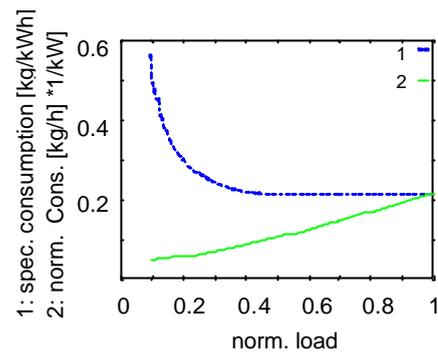
Fig. 1: Characteristics of the fuel consumption of a diesel generator set DGS. Given are the absolute (lower curve) and specific fuel consumption in dependence of the diesel loading. Both the load and the fuel consumption are given in a form normalized to the nominal power output of the system. Data are taken from manufacturers data sheets (Anonymous 2002).
