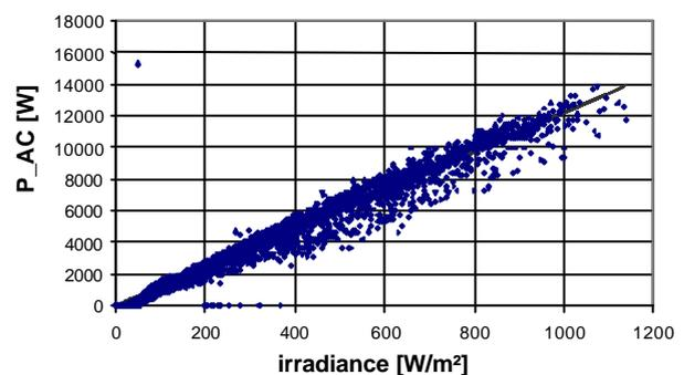
Fig. 7: AC-performance of the PV generator at Araras. The actual performance of the generator (nameplate rating 21 kW) is equivalent to a rating of about 12.5 kW.
