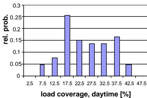
Fig. 9: Distribution of the daytime load coverage by PV in the Araras system. The average is at about 20%.
