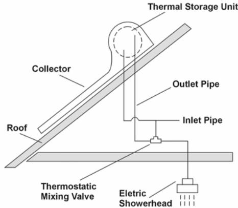
Figure 1. Compact solar hot-water system scheme
