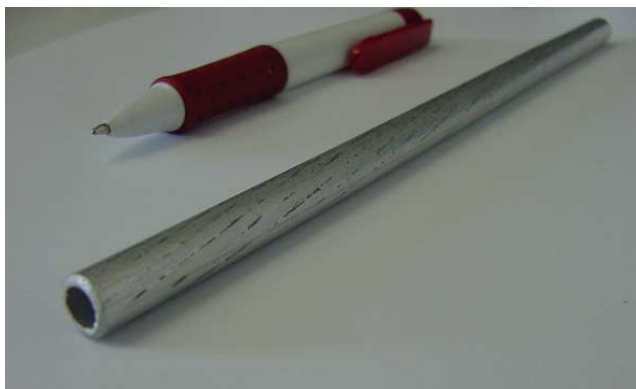
Figure 1. Aluminum tube of the OPGW
