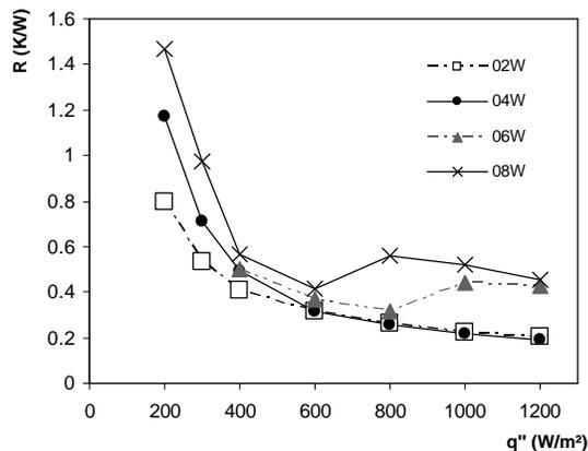
Figure 5. Overall thermal resistance of TPCTs as a function of the heat flux for water as working fluid and no helicoidal wire.
