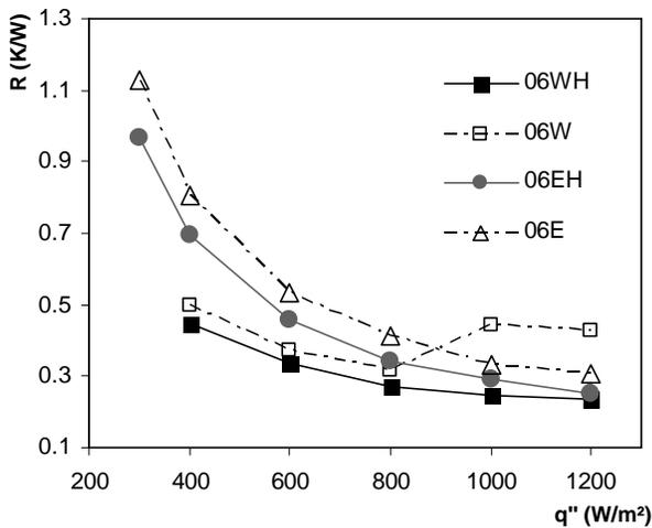
Figure 8. Overall thermal resistance of TPCTs as a function of the heat flux with filling ratio equal to 0.6.
