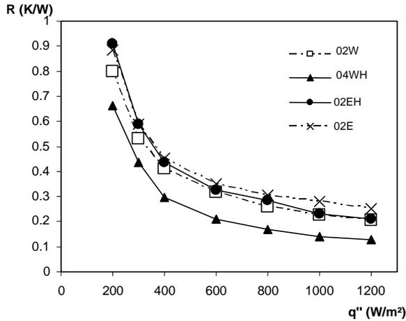
Figure 7. Overall thermal resistance of TPCTs as a function of the heat flux for the best case scenarios for either water or ethanol as working fluid and with or without the helicoidal wire.
