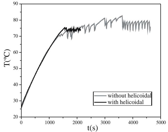
Figure 3. Start-up evaporator temperatures of TPCTs with filling ratio equal to 0.6, water as working fluid and heat flux equal to 400 W/m<sup>2</sup> (67.5 W).
