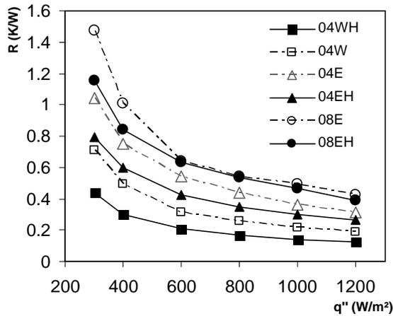
Figure 4. Overall thermal resistance of TPCTs as a function of the heat flux showing lower thermal resistances when the helicoidal wire is present.
