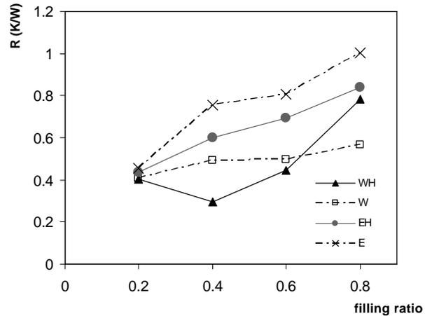
Figure 6. Overall thermal resistance of TPCTs as a function of the filling ratio for all TPCTs, with heat flux equal to 400 W/m<sup>2</sup> (67.5 W).
