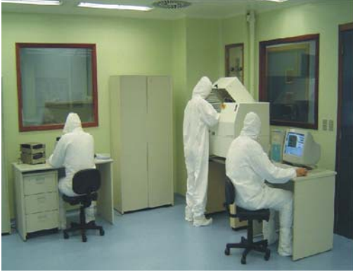
Fig. 3: Clean room facilities (190 m 2 , 10.000 class, ISO 7) designed to produce silicon solar cells and PV modules.
