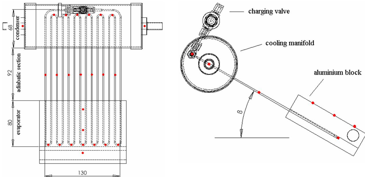
Figure 1. Experimental apparatus showing the thermocouple distribution (red dots).
