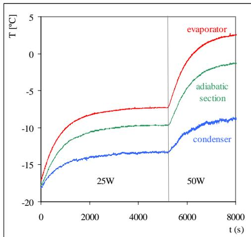
Figure 4. Transient variation of the average evaporator temperature for FR=50% and  $\beta=90^\circ$ .
