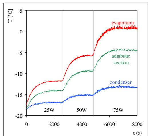
Figure 3. Transient variation of the average evaporator temperature for FR=50% and  $\beta=45^\circ$ .
