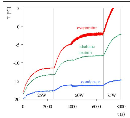
Figure 2. Transient variation of the average evaporator temperature for FR=50% and  $\beta=0^\circ$ .
