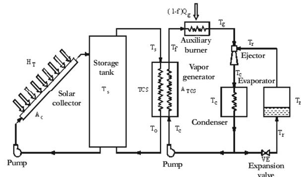
Fig 1: Solar assisted ejector cooling system.
