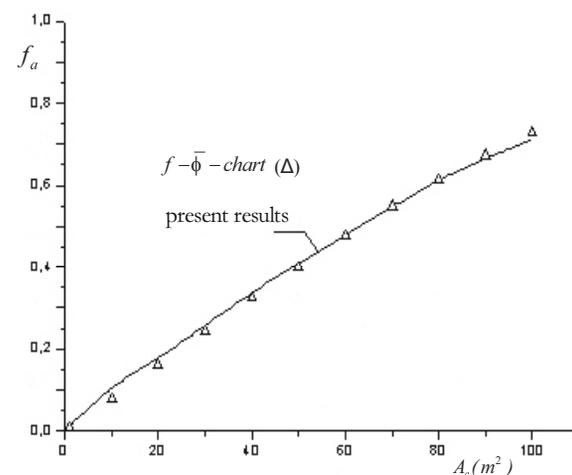
Fig. 2: Plots of  $f - \bar{\phi}$  - chart results for  $T_{min} = 77^\circ\text{C}$  against results for the annual fraction  $f_a$  for  $A_{TCS} = 3$  m<sup>2</sup>.
