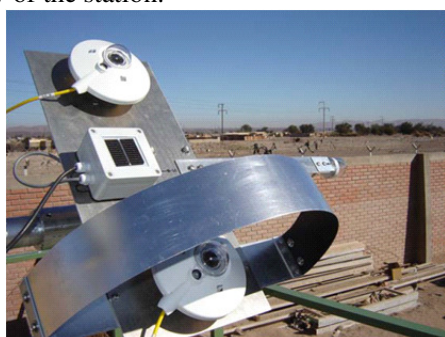
Figure 3: View of the CNE-GTZ station, detailing the pyranometers used in the “tracking” mode (left). Summary of data produced by the station (right).
