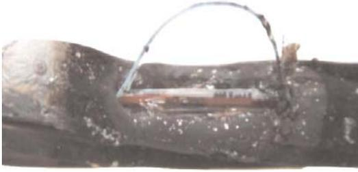
**Figure 2. OPGW cable damaged by lightning**
