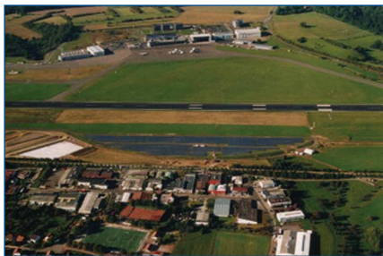
Figure 3: Saarbrücken Airport (Germany) showing the 1.4MWp ground-mounted PV installation operating since 2004
