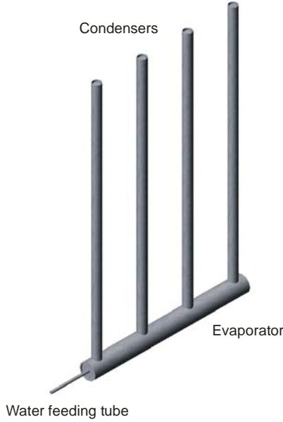
Figure 1. Schematic of the tree configuration thermosyphon
