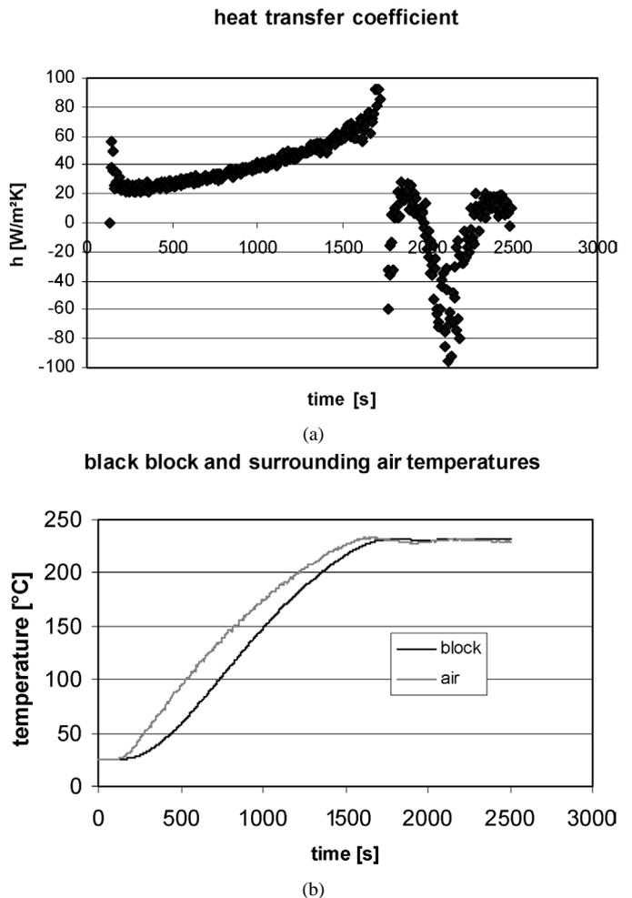
Fig. 11. Measured heat transfer coefficient versus time (a). Measured temperatures of a typical black block and surrounding air during transient (b).
