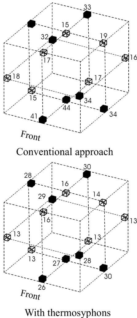
Fig. 10. Distribution of heat transfer coefficients inside the enclosure under steady state [ $W \cdot m^{-2} \cdot K^{-1}$ ].
