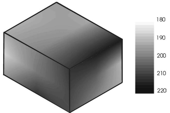
Fig. 6. Temperature map inside the enclosure heated using the conventional approach.
