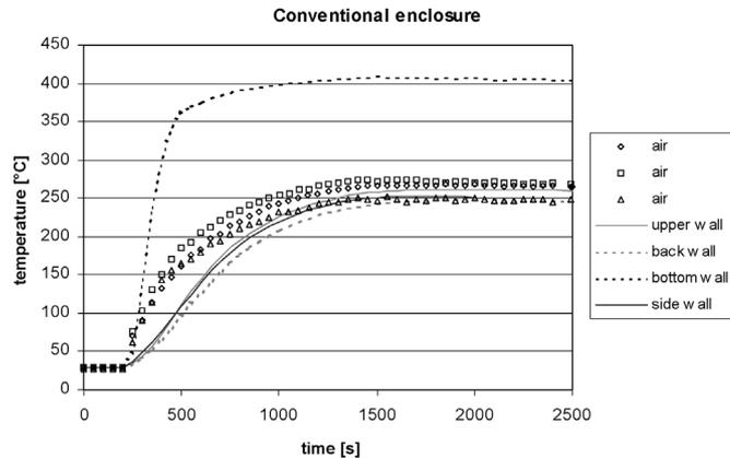
Fig. 8. Measured temperature variation with time during start-up for the conventional enclosure.
