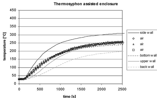
Fig. 9. Temperature variation with time during start-up for the thermosyphon assisted enclosure.
